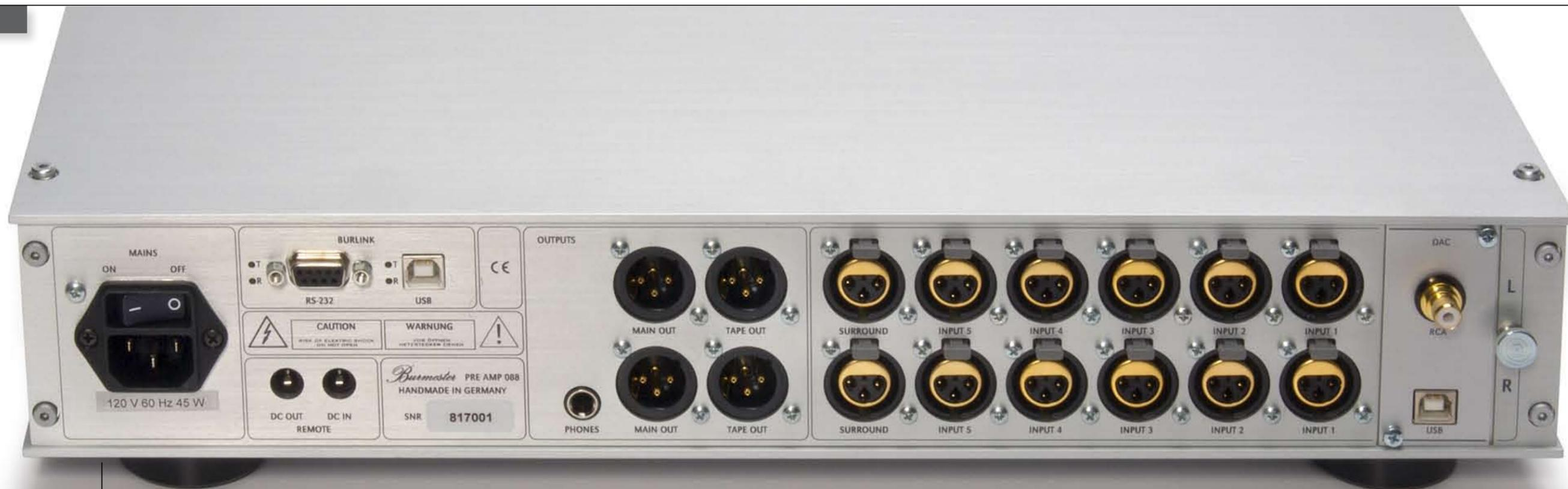
**While older preamplifiers like the 011 boast a few unbalanced inputs and a pair of unbalanced variable outputs, the 088 is balanced throughout and utilizes XLR inputs and outputs.**
