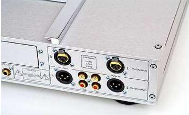
*Proven concept: Although the 089 is also receptive for RCA connections, the greatest sound potential lies at the balanced outputs.*
