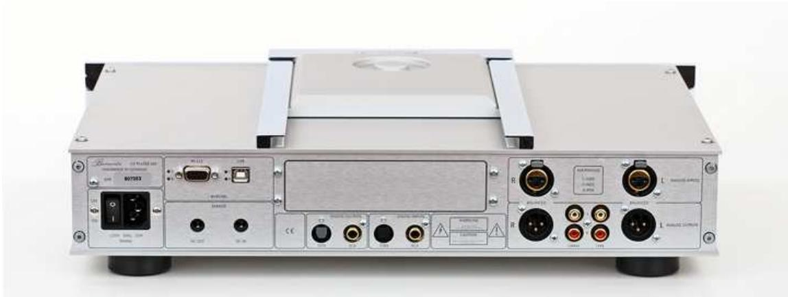
*Tidy command centre: besides the required outputs the Burmester 089 CD player has several inputs, too. It offers USB and RCA and of course XLR inputs. Since it is equipped with high-class preamp, this player may also double as the heart of a small, but very fine high-end system.*
